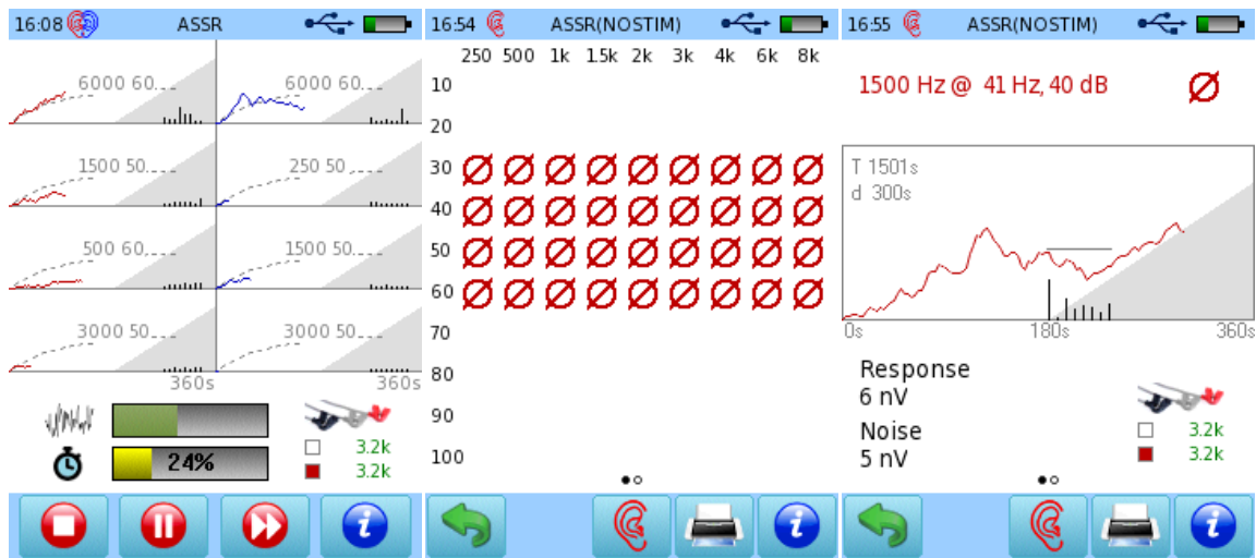
Fig. 3: Test results with Spread Spectrum enabled, recording contaminated EEG test signal. Left panel: ongoing test, with the 1500 Hz 50 dB channel not detecting any response. Mid panel: Overall result for right ear (no response was detected on the left ear). Both frequencies that used 41.25 Hz average stimulus rate now are free from false responses. Right panel: Single result (1.5 kHz, 41.25 Hz, 40dB) with no statistically significant response.
