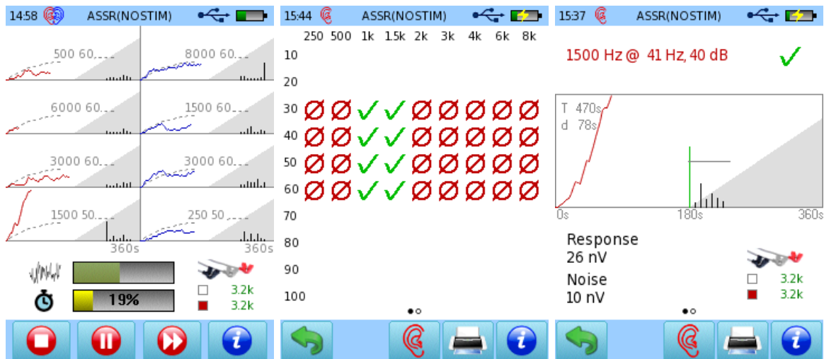
Fig. 2: Test results without Spread Spectrum, recording contaminated EEG test signal. Left panel: ongoing test, with the 1500 Hz 50 dB channel obviously recording a false response. Mid panel: Overall result for right ear (no response was detected on the left ear). Both frequencies that used 41.25 Hz stimulus rate produced false detections. Right panel: Single result (1.5 kHz, 41.25 Hz, 40dB) with a strong false response. A real ASSR response would look quite similar.
